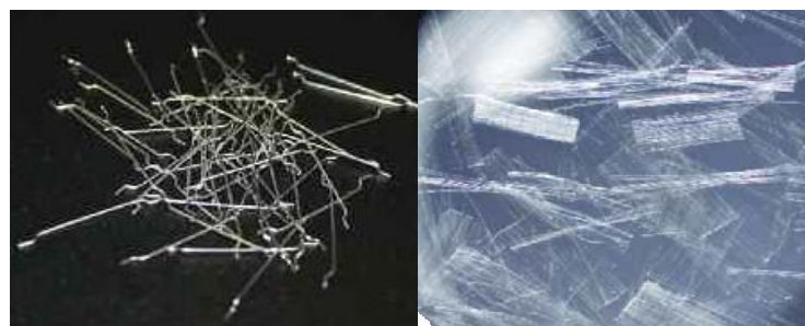
Figure 1: Hooked steel fiber 30mm length, Polypropylene FIBERMESH® 30012mm length
