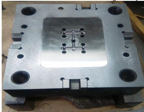
Fig. 5. The assembly process of the eight-cavity mold for injection molding of MIM 4140 alloy.
