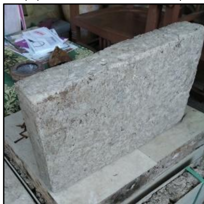
Figure 10 Soil-paper blocks without calcium silicate panels (WP)
