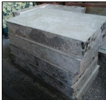
Figure 9 Soil-paper block with calcium silicate panels
