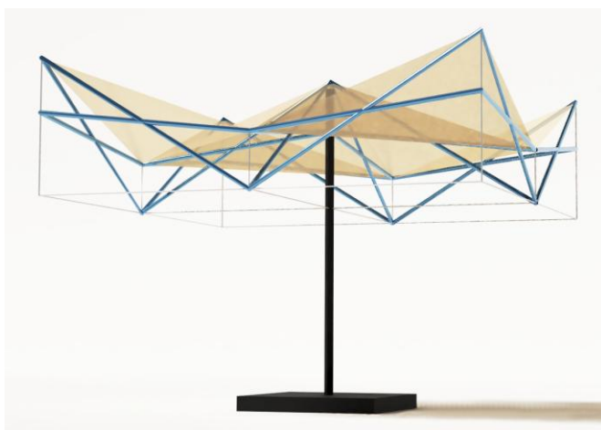
Figure 10. Expandable umbrella with square modulus
