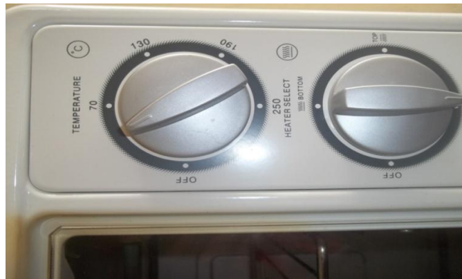
Temperature and drying time (45 0 C, 9 hours)
